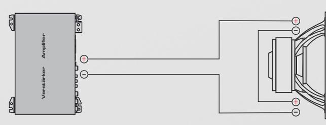
2 Subwoofer Parallel/Serial wiring: 2 Ohm
